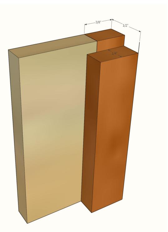
The door and pull are not fully shown. This view is intended to show how the door and pull are assembled. See video for technique for getting a good fit.
